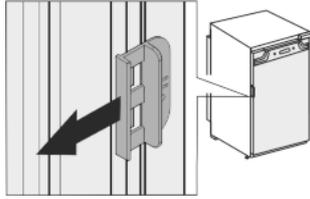
If the transport lock is screwed onto the door:
