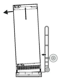
Slide a transport dolly between the appliance and packaging. Tie the appliance to the dolly with straps. Tilt the appliance onto the dolly.
