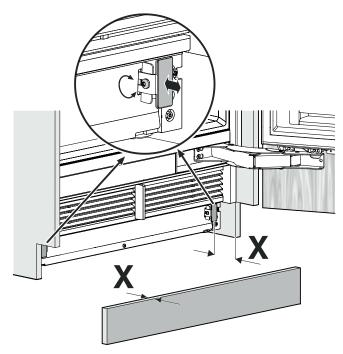
Remove the backing foil and affix the plinth panel.
