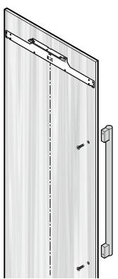
Only use countersunk screws for handle mounting.
