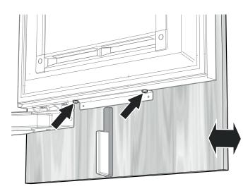
Secure the panel through the bottom attachment bracket with two 4 x 14 screws.
