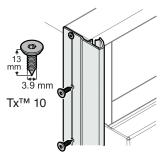
Apply the appliance cover strips to the left and right front edge of the appliance housing, align in height with the appliance top and screw into place. The strip is transparent so that the designed attachment holes on the appliance housing are visible. We recommend that you mark and pre-drill the hole positions in the strip.
