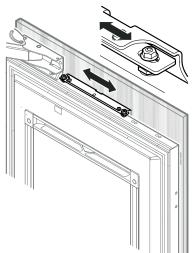
Align the panel horizontally with the long slots in the attachment bracket.
