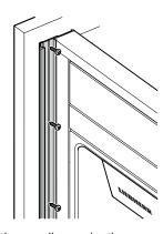
Fasten the appliance in the recess through the appliance cover strips using eight 4 x 14 mm screws for each side. We recommend that you mark and pre-drill the hole positions in the strip.
