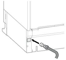
Pull the water line through from the rear to the front.
