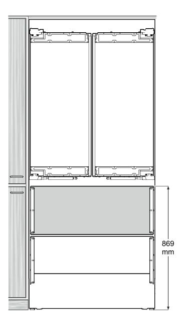
Adjust the appliance in the recess to a **reference height** of **869 mm**, measured from the floor to the top of the upper freezer drawer.
