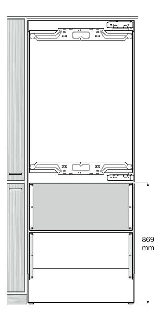
Adjust the appliance in the recess to a **reference height** of **869 mm**, measured from the floor to the top of the upper freezer drawer.
