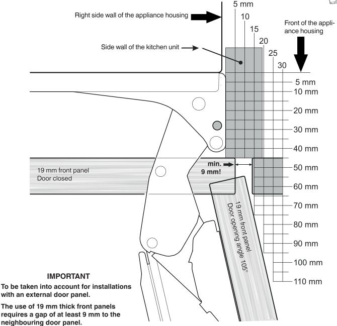
If the gap is less than 9 mm, the front vertical edge of the door panel will collide with the front vertical edge of the neighbouring panel when the door is opened.
