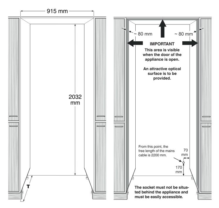
Recess depth  ${f T}$  for installations with external door panel = 610 mm
