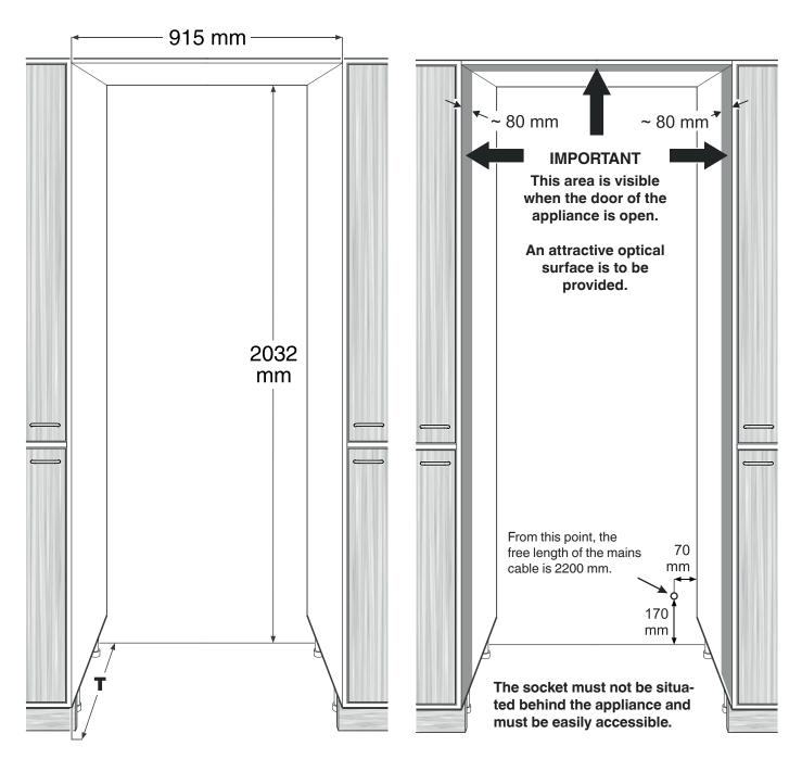
Recess depth **T** for installations with external door panel = 610 mm
