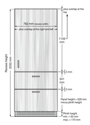
Minimum panel thickness = 16 mm Maximum panel thickness = 19 mm
