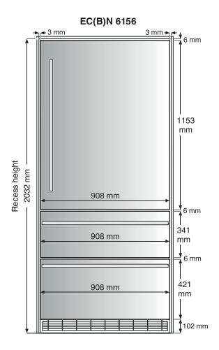
Appliance dimensions (height dimensions are with adjustable feet or castors fully screwed in)
