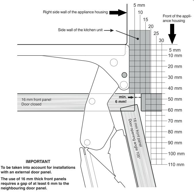
If the gap is less than 6 mm, the front vertical edge of the door panel will collide with the front vertical edge of the neighbouring panel when the door is opened.
