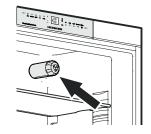
If the water pressure with the inserted water filter is too low, this may cause the IceMaker to malfunction.
