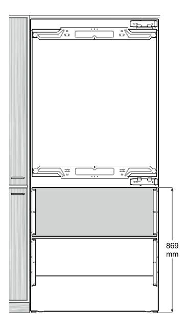
Adjust the appliance in the recess to a **reference height** of **869 mm**, measured from the floor to the top of the upper freezer drawer.
