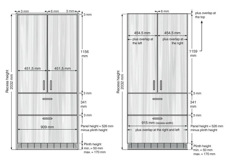
Minimum panel thickness = 16 mm Maximum panel thickness = 20 mm
