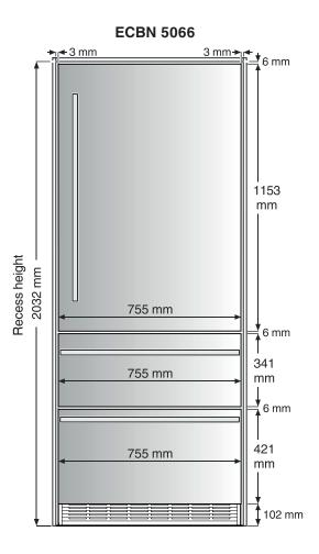
Appliance dimensions (height dimensions are with adjustable feet or castors fully screwed in)
