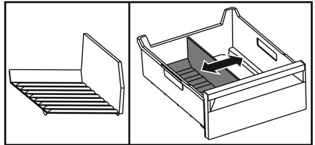
Fig. 119 Example illustration of the ice compartment divider
