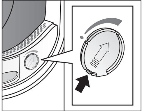
If you are not using a fragrance flacon: push the tab down completely (see arrow) so that the socket is closed. Otherwise, lint will accumulate here.
