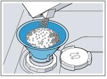
Fill the dispenser right up with special salt. The water in the dispenser is displaced and forced out. 4. Place the lid back on the dispenser and turn to close.
