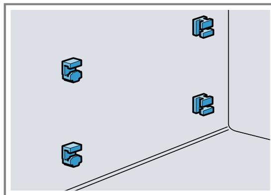
1. Hook the front retainers with the hook into the round hole at the top and set them at a slight angle  $\textcircled{1}$ .
