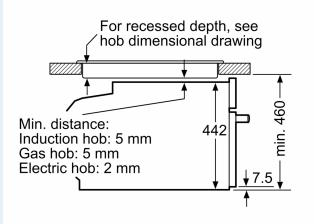
If the compact appliance will be installed underneath a hob, the following worktop thicknesses (including substructure if necessary) must be taken into acccount.
