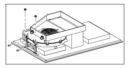
■ Undo the fixing brackets.
