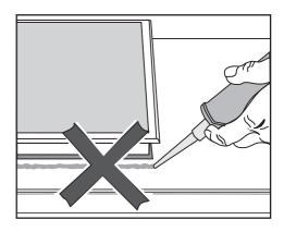
Damage caused by incorrect installation.
