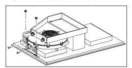
■ Undo the fixing brackets.
