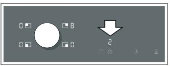
To set a different fan setting, touch the Symbol and use the twist knob to select the required setting.
