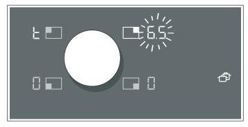
3 Use the twist knob to select the new hotplate within 90 seconds. The setting has been transferred.
