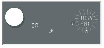
The appliance tries to connect to the app automatically.  $H_{L}^{c}$  and  $P_{R}^{c}$  i flash alternately in the settings area. The  $\square \square$  value flashes on the hotplate display.
