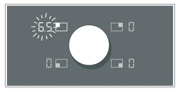
2 Set the cookware down on a flexible hotplate within the next 90 seconds. The new hotplate will be detected and the <sup>1</sup>/<sub>1</sub> symbol will light up. The applied heat setting will flash in the hotplate display.
