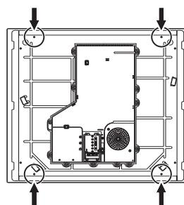
2. Fasten the fixing brackets (A) into the holes marked using the screws that
